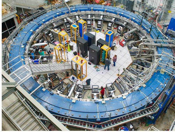
Fig. 1. The E989 storage ring at Fermilab, which was originally designed for the E821 experiment. Superconducting magnets provide a uniform radial magnetic dipole field of 1.45 T. The 24 calorimeters are shown distributed uniformly on the inside of the ring. The beam (shown in red at the top of the figure) enters the storage ring via the inflector. The direction of the beam is clockwise in this orientation.
